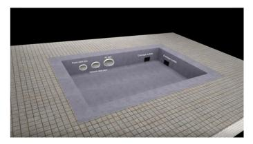
2. Fans must be installed at the air inlet and outlet.
