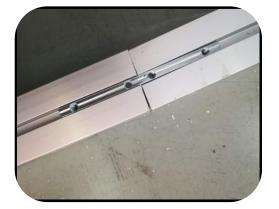
2. Place the positioning columns of the cabinet on the positioning hole of the guide rails,
