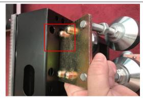
5. Adjust the screw height so that the screen is at the same level.
