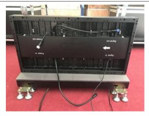
9. Connect the power cable and the network cable in order.
