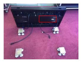
4. Place the positioning hole of the floor screen on the positioning column of the floor support.
